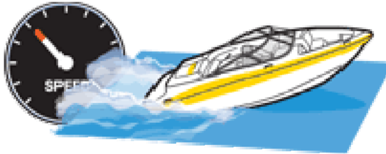
Figure 5 Hull in Plowing Mode
